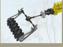
HEAVY DUTY DRIVE LINE (HDDL) » The HDDL is developed for the hardest of applic cations and is very robust. The attachment is driven by a fixed PTO shaft, and still has
